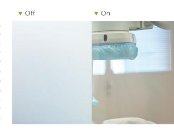
Smart Film displays a foggy state when it is not charged with electricity, when alternating current, the internal liquid crystal molecules will appear in an orderly manner, at this time, the Smart Film will turn transparent from its original foggy state. Through the on and off switch on the alternating current makes it easy to quickly transform the state of the Smart Film from transparent to opaque.
