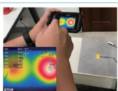
A By conducting actual experiment, heating LOFANS energy saving brick (Left) and normal generalized brick (Right) for 100 minutes, the temperature difference could be up to 15 degrees Celsius, which could effectively reduce the indoor temperature within the building.
